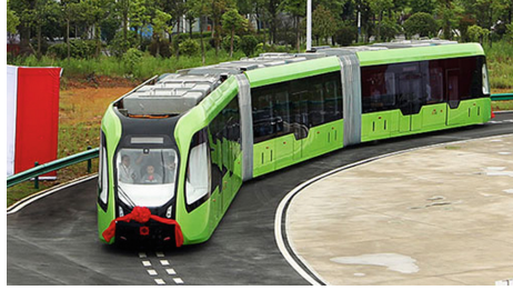
Fig. 1. A 3-unit Autonomous rail rapid transit vehicle on the track.
